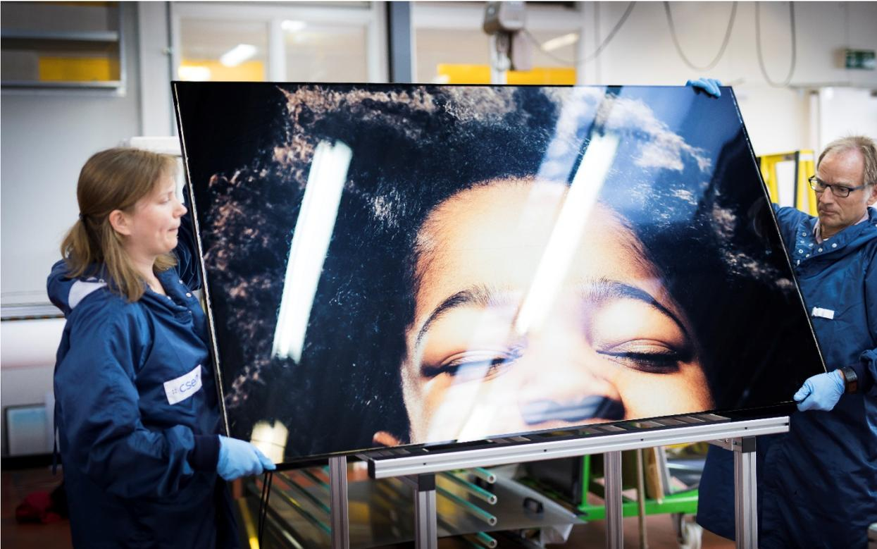
*The image is printed on a film that has been specially chosen to be durably integrated in the solar module.*
